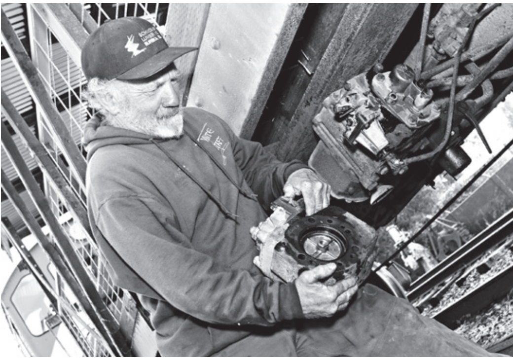
Chris Baldo after changing the service portion of the AB brake valve on the Sacramento Northern 1638 riding car.
