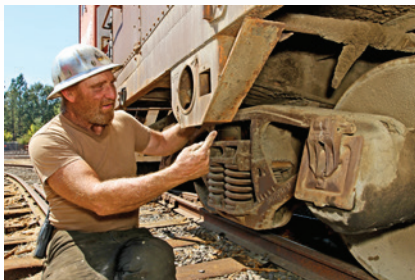
Above: Roots of Motive Power's Troy James shows features of the newest yard inhabitant: the Pacific Fruit Express Car, a refrigerator box car which has insulated walls “this thick,” left, which was cooled with blocks of ice at each end. Fans on each end of the car circulated the cool air and were powered by friction-driven generators, mounted where James points, right, on each car.
