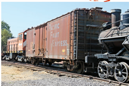
Above: Roots of Motive Power's Troy James shows features of the newest yard inhabitant: the Pacific Fruit Express Car, a refrigerator box car which has insulated walls “this thick,” left, which was cooled with blocks of ice at each end. Fans on each end of the car circulated the cool air and were powered by friction-driven generators, mounted where James points, right, on each car.
