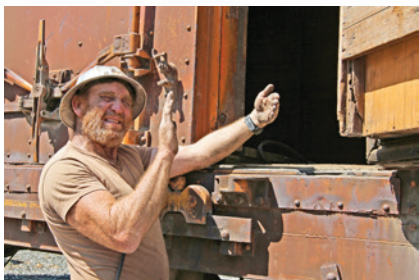
Above: Roots of Motive Power's Troy James shows features of the newest yard inhabitant: the Pacific Fruit Express Car, a refrigerator box car which has insulated walls “this thick,” left, which was cooled with blocks of ice at each end. Fans on each end of the car circulated the cool air and were powered by friction-driven generators, mounted where James points, right, on each car.
