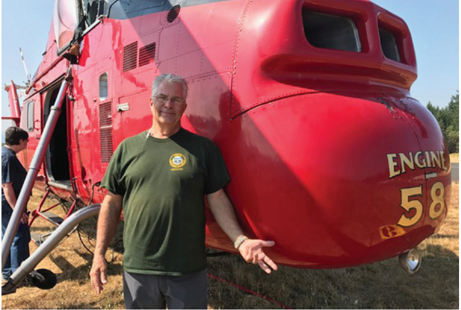
At right, top: Capt. Roger Caballero, right, stands with the pilot of the Sikorsky Skycrane, a water-dropper owned by Siller Helicopters out of Yuba City. The Skycrane has a 2,650 gallon capacity water tank, which uses a hydraulically driven boat propeller at the end of a 25-foot snorkel hose to sip up water or retardant and can sit tank in as little as 45 seconds. At right: Pilot Steve Bull stands in front of the Sikorsky 58T, a two-seater, single-pilot helicopter, which has a two turbine engine, and was built in 1958. Bull and his crew fly for ARIS Helicopters out of Corona and Hollister, and are a "call when needed" crew, consisting of the pilot, a crew mechanic and a field truck trucker. The Sikorsky is a water-dropper using a 350 gallon Bambi Bucket, but can also bring cargo and food in and out of a fire site.
