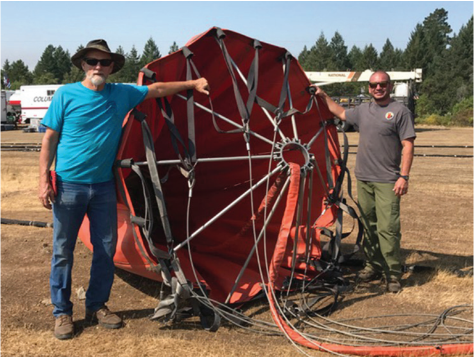
At right: John Wagenet and Capt. Roger Caballero from Tahoe Helitack, stand next to a large Bambi Bucket. The bucket dips into water sources such as lakes, ponds and creeks, then expands with the water to form the ball shape seen dangling from 100-foot-long lines attached to firefighting helicopters.
