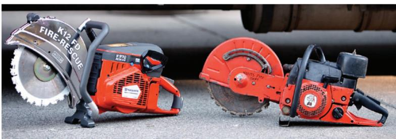
it to cut through anything from concrete to metal to shingles and comp roofs. Typically a rotary saw is used for vertical ventilation to help prevent back draft, allowing the superheated gas to escape through a hole cut into the structure's roof. LLFD firefighters noted this is a common procedure, used on about 50 percent of their calls.
